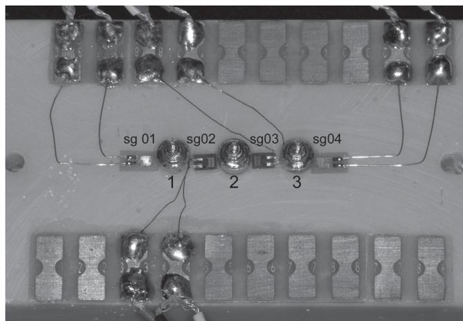
Fig. 2 - Strain gauges around the microunit abutments.
