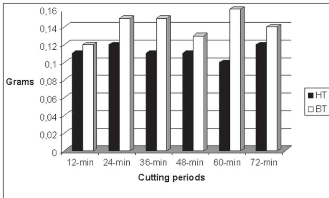
Fig. 2. Mean mass loss values (in g).
