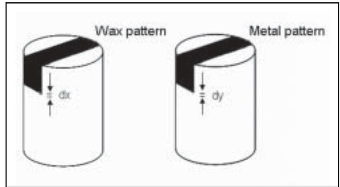
Fig. 1. Dimensional accuracy of a cast crown expressed by the discrepancy measured on its wax pattern (dx) and coating (dy) on the same die.
