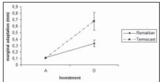
Fig. 2. Marginal discrepancies of the cast MOD titanium inlays invested with Rematitan Plus' and Termocast'. Each line represents the means and standard deviation before (A) and after (B) casting.
