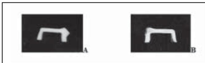
Fig. 3. Radiographic images of a titanium inlay cast with Rematitan Plus<sup>®</sup> (A) and Termocast<sup>®</sup> (B).
