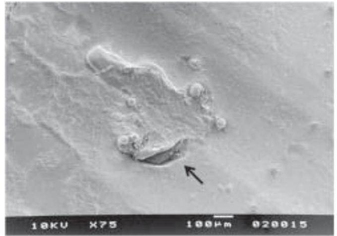
Figure 2. Group 2 (Resilon™). SEM micrograph of a tooth subjected to apicoectomy after root canal filling with Resilon™ cones. Arrow indicates to gap areas ( $\times 75$  magnification).
