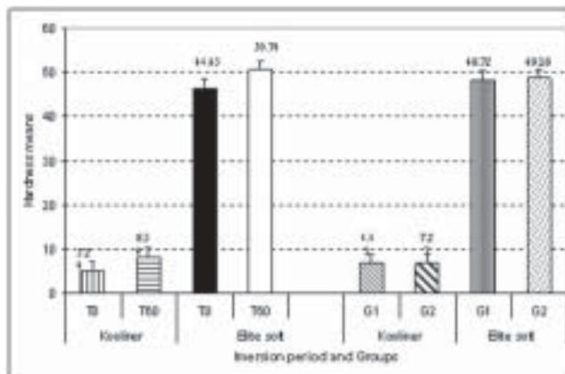
**Fig. 2 - Hardness means and standard deviations of the tested materials.**
