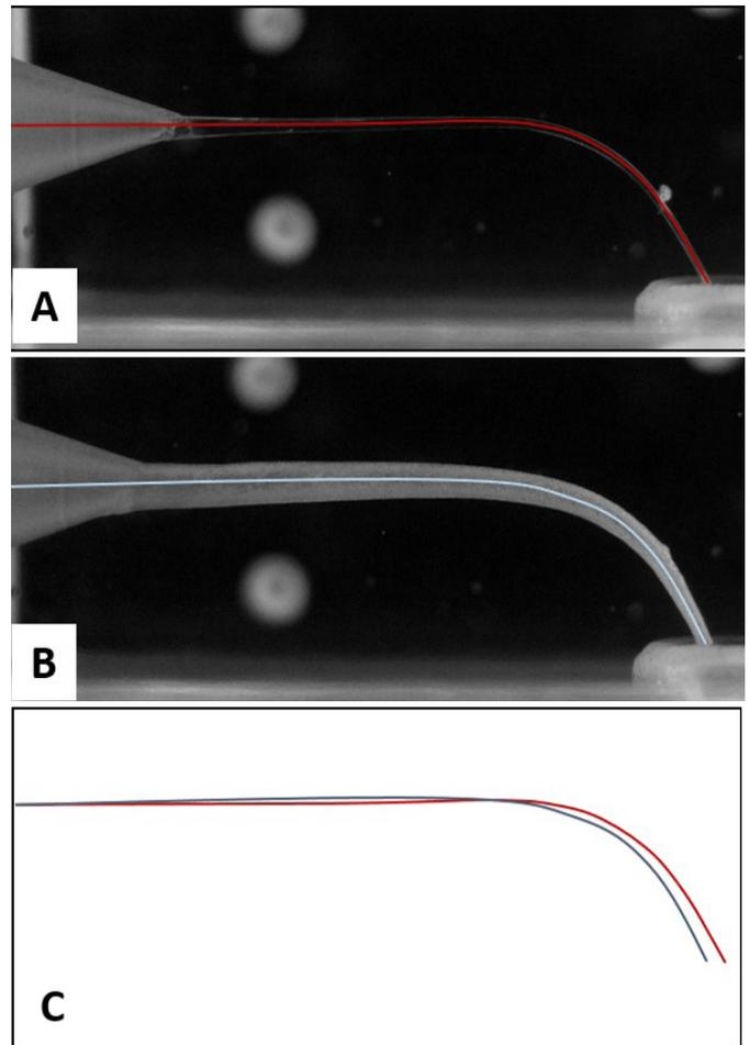
**Fig. 1** - Image of a simulated canal block taken before (A) and after (B) preparation and corresponding centerlines obtained after the analysis. (C) Superposition of baseline and final centerlines showing that transportation occurred after instrumentation.
