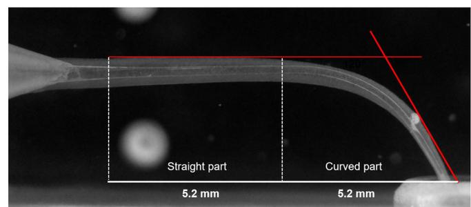
**Fig. 2** - Determination of straight and curved parts of one simulated canal before and after instrumentation.
