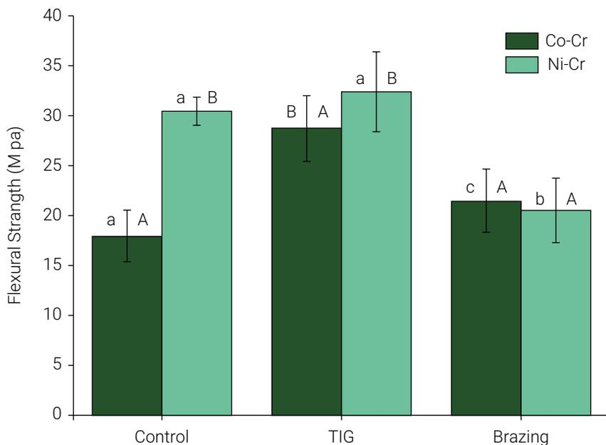
**Figure 3.** Mean flexural strengths (MPa) in the control, TIG, and brazing groups based on the different welding and framework types. The different lower case letters represent significant differences among the same type of alloy associated with the different types of welding methods used. The capital letters represent significant differences among the different structures related to the same of type welding method used.
