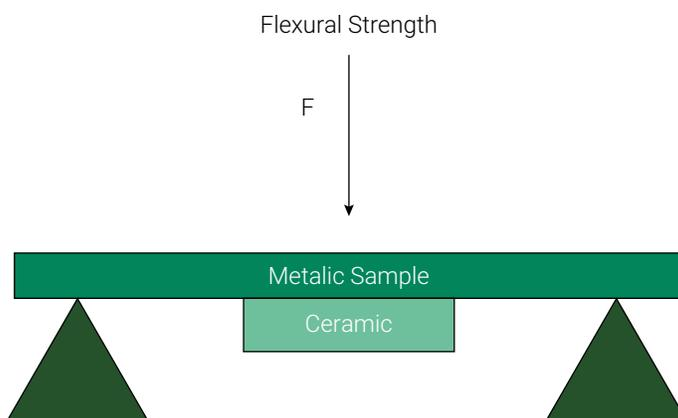
**Figure 2.** Flexural Strength assay
