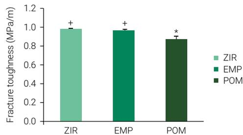
**Figure 3.** Results of fracture toughness (MPa/m) of the ceramics evaluated. Different symbols represent statistically significant difference ( $\alpha=5\%$ ).
