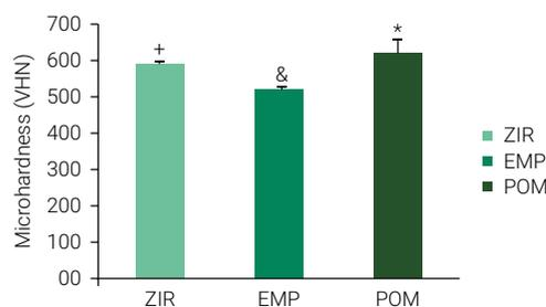
**Figure 1.** Results of Vickers microhardness (VHN) of the ceramics evaluated. Different symbols represent statistically significant difference ( $\alpha=5\%$ ).
