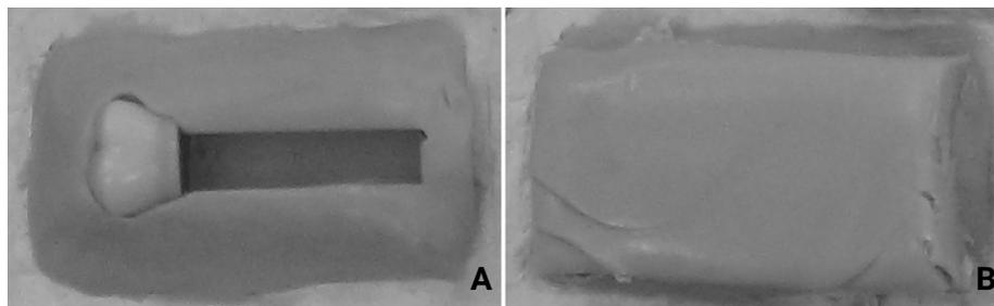
**Figure 1.** Initial preparation of samples. A) The artificial tooth was put into the silicone layer. B) Another layer of silicone covered the tooth. After stone set, the acrylic resin was included on the hole in silicon
