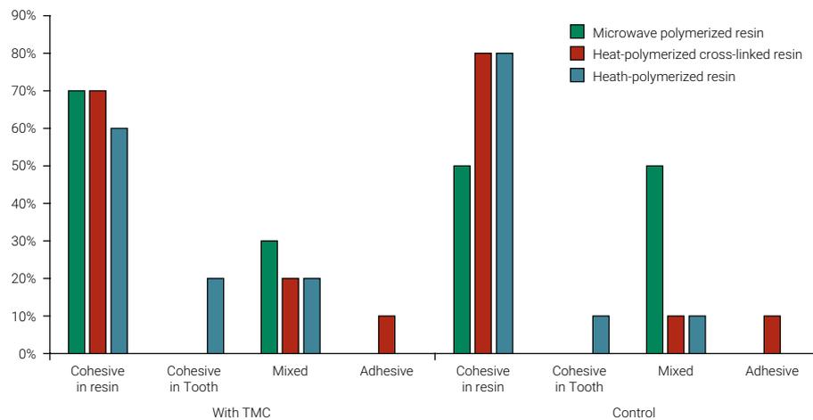
**Figure 3.** Distribution, in percentage, of the fracture types for each group. (TMC = Thermomechanical cycling)
