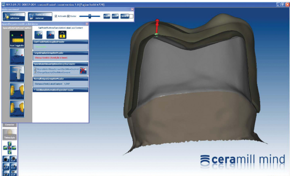
Figure 1. Example of the core with 1.0 mm thickness at occlusal face designed in the Ceramill Mind software
