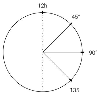
**Figure 1.** Description of the directions considered for measuring the surface roughness.
