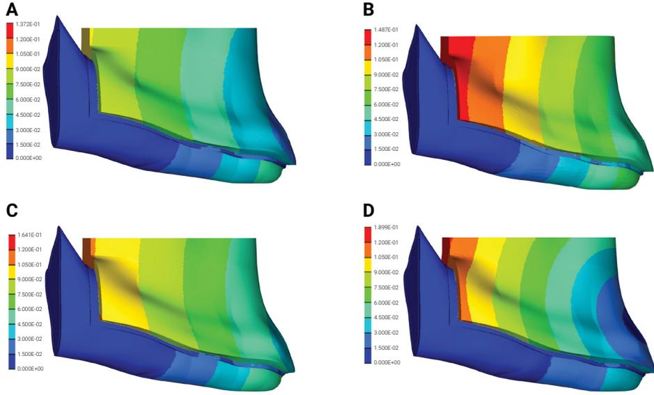
**Figure 4.** Stress maps (Displacement) combined in the overdenture and jaw. A, Group C-0°. B, Group C-17°. C, Group LI-0°. D, Group LI-17°. Color stress scale in MPa. C-0°, implant positioned in the canine region 0° to the vertical axis. C-17°, implant positioned in the canine region 17° to the vertical axis. LI-0°, implant positioned in the lateral incisor region 0° to the vertical axis. LI-17°, implant positioned in the lateral incisor region 17° to the vertical axis.
