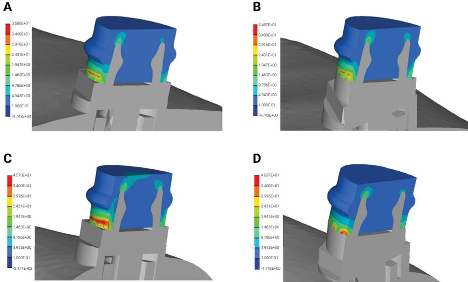
**Figure 6.** Stress maps (von Mises stress) on Micro ERA® nylon. A, Group C-0°. B, Group C-17°. C, Group LI-0°. D, Group LI-17°. Color stress scale in MPa. C-0°, implant positioned in the canine region 0° to the vertical axis. C-17°, implant positioned in the canine region 17° to the vertical axis. LI-0°, implant positioned in the lateral incisor region 0° to the vertical axis. LI-17°, implant positioned in the lateral incisor region 17° to the vertical axis.
