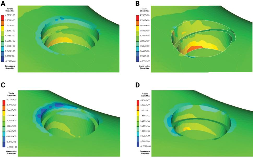
**Figure 5.** Stress maps (compressive/tensile stress) on implant/bone interface. A, Group C-0°. B, Group C-17°. C, Group LI-0°. D, Group LI-17°. Color stress scale in MPa. C-0°, implant positioned in the canine region 0° to the vertical axis. C-17°, implant positioned in the canine region 17° to the vertical axis. LI-0°, implant positioned in the lateral incisor region 0° to the vertical axis. LI-17°, implant positioned in the lateral incisor region 17° to the vertical axis.
