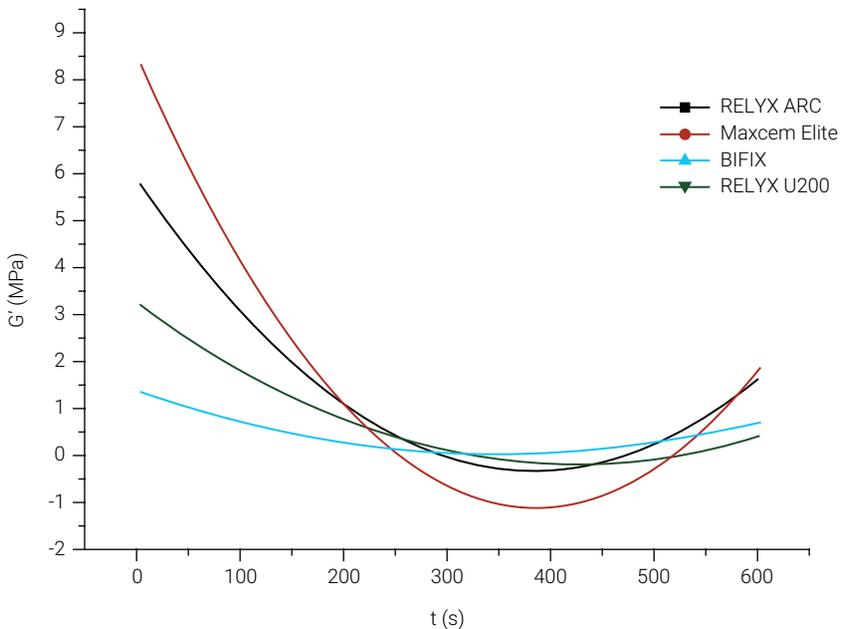
**Figure 1.** Rheological behavior of the four cements analyzed. EM(MPa) and time in seconds(s)
