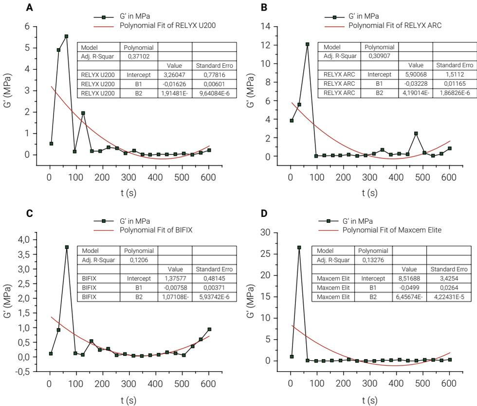
**Figure 2.** (A) Rheological behavior of RelyX U200 cement. EM(MPa) and time in seconds(s); (B) Rheological behavior of RelyX ARC cement. EM(MPa) and time in seconds(s); (C) Rheological behavior of Bifix SE cement. EM(MPa) and time in seconds(s); (D) Rheological behavior of Maxcem Elite cement. EM(MPa) and time in seconds(s)
