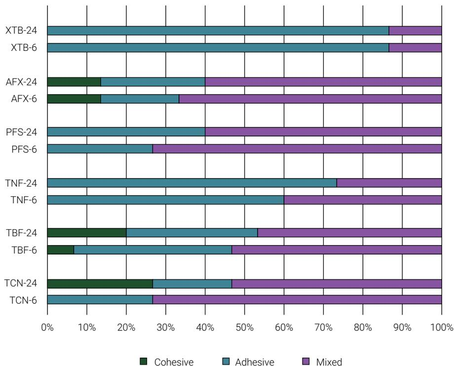
**Figure 3.** Distribution of the failure modes according to the resin composite and aging time analyzed. Column: aging time to perform the test (24 - 24h or 6 - 6 months) after specimen preparation. Lines: % of the failure modes. TNF: Tetric N-Ceram; TBF: Tetric N-Ceram Bulk fill; TNF: Tetric N-flow; PFS: Polofil Supra; AFX: Admira Fusion X-tra; XTB: X-tra Base.
