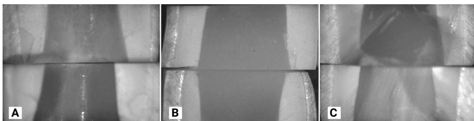
**Figure 2.** Failure modes obtained in this study: Adhesive (A), Cohesive (B), Mixed (C).
