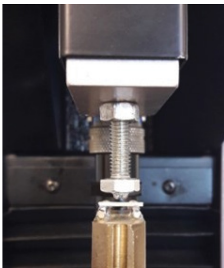
Figure 1. Example of a beam accordingly positioned between the supports for the flexural bond strength assay.
