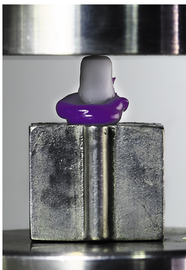
Figure 3. Zirconia coping cementation with silicone in universal testing machine.
