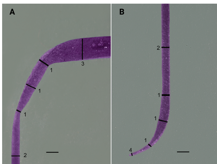
Figure 6. Standardization (original magnification ×100) used to measure the regions misfit. A: angular (1), linear (2), and incisal regions (3). B: angular (1), linear (2) and marginal regions (4). Perpendicular line drawn from abutment to internal surface of coping. Scale bar, 100 μm.
