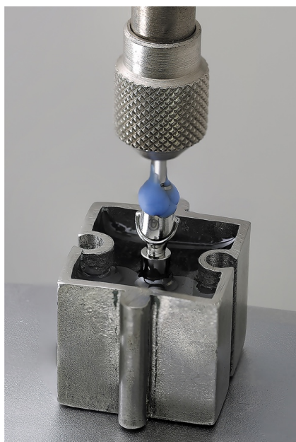
Figure 1. Anatomic titanium abutment on implant analog fixed to metal parts.
