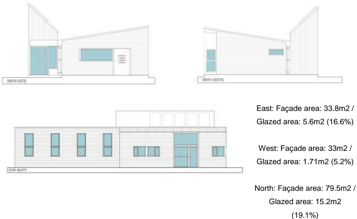
Figure 12 East, West and North elevations with their glazed surfaces highlighted
