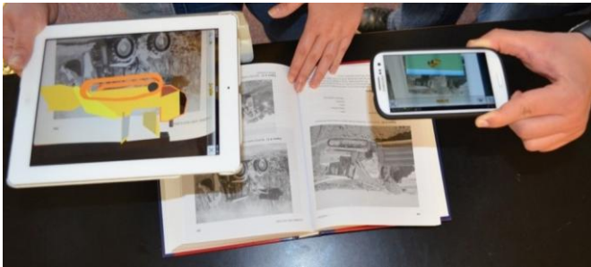
Figure 3 - Two users simultaneously viewing virtual contents overlaid on two different pages of the textbook
