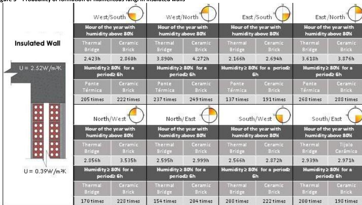
Figure 5 – Probability of formation of filamentous fungi in insulated walls
