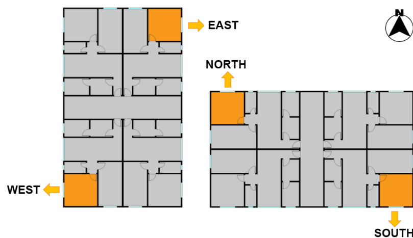
Figure 2 - Floor plan with the positioning of the simulated environment in relation to the openings
