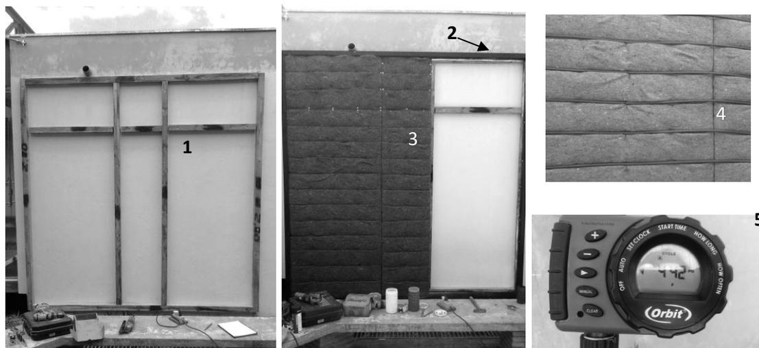
Notes: 1. Rafters, 2. Seal and drainage gutters, 3. Eco-plate modules with geotextile layers and 4 and 5. Irrigation lines and controller. Source: the authors.
