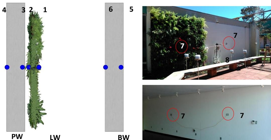
Notes: PW: protected wall; LW: living wall; BW: bare wall/control plot. 1-Tsej; 2- Tsij; 3- Tsepp; 4-Tsipp; 5- Tsepc; 6- Tsipc; 7- Sensors for monitoring surface temperatures; 8- Net-radiometer. Source: the authors.
