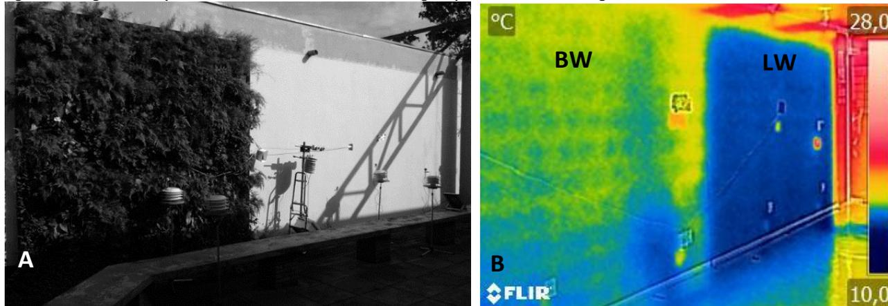
Notes: A- Experimental field at 9:15 am with solar incidence in the plots. B- Internal surfaces of the plots with and without garden at 11:45 am. LW: living wall; BW: bare wall. Source: The Authors.
