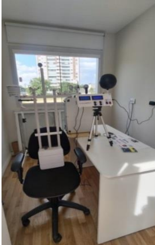
Figure 4 – Interior of the CBC bioclimatic chamber with PLEMS and the reference equipment
