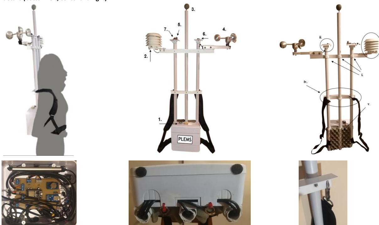
Figure 2 – Details of the backpack attachment to the user (top left), location of the sensors (top center and top right) and PLEMS construction details (bottom left, center and right)
