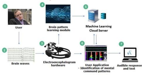
Figure 8. Software architecture.
