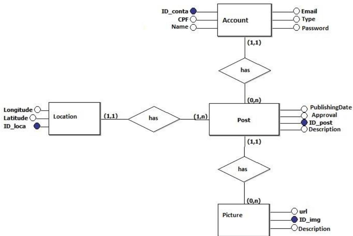
**Figure 2 - Entity Relationship Model for Urban Flooding App.**
